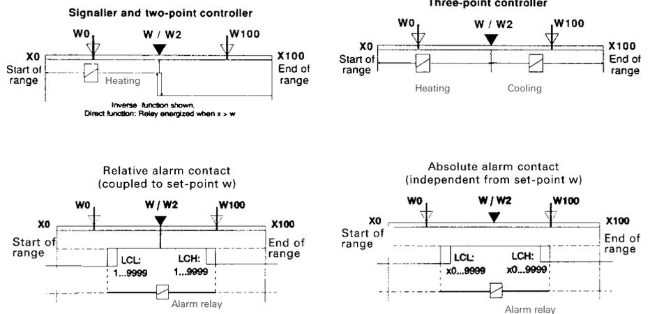
Upper and lower alarm can be disabled, and switching difference  $S_d$  is adjustable. On alarm, relay is energized (as shown), and logic output = 1. Functions are valid for relays 1 and 2.
