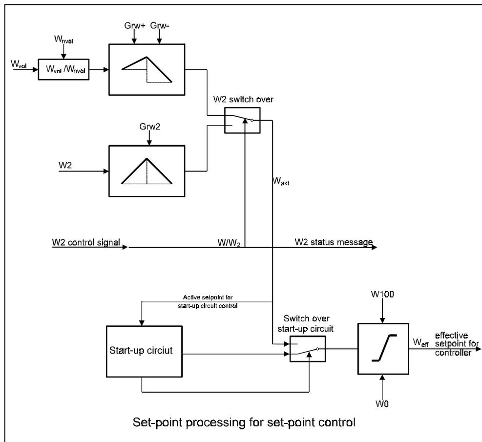
The effective set-point for KS 816 undergoes various pre-processings, before it is used for the control algorithm.
