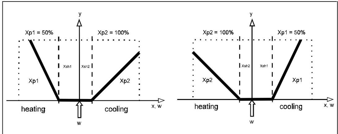
The static characteristic for inverse and direct output action with  $T_n = 0$  is shown in the figures. Direct/inverse switch-over only causes an exchange of the outputs for „heating/cooling“.
