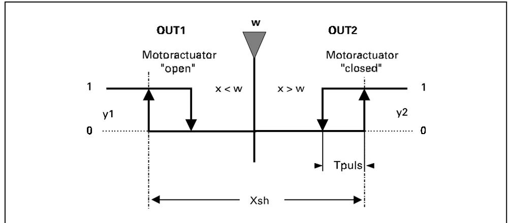
**Configuration example: room temperature control by means of a motor-actuated valve.**
