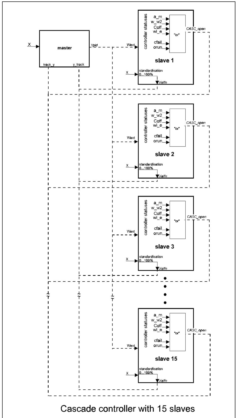
For special applications, connection of up to 16 slave controllers to a master can be necessary. In this case, the master controller correcting variable is used as slave controller set-point. The slaves control the connected loop individually with the adjusted parameters.
