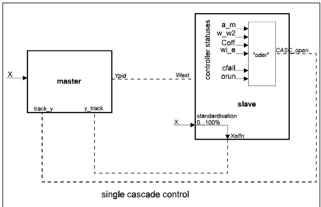
In the example shown above, 4 groups each with one master and one slave are possible. The controllers of a cascade are connected internally via configuration and communicate with each other. Additional input and output scaling is not necessary.
