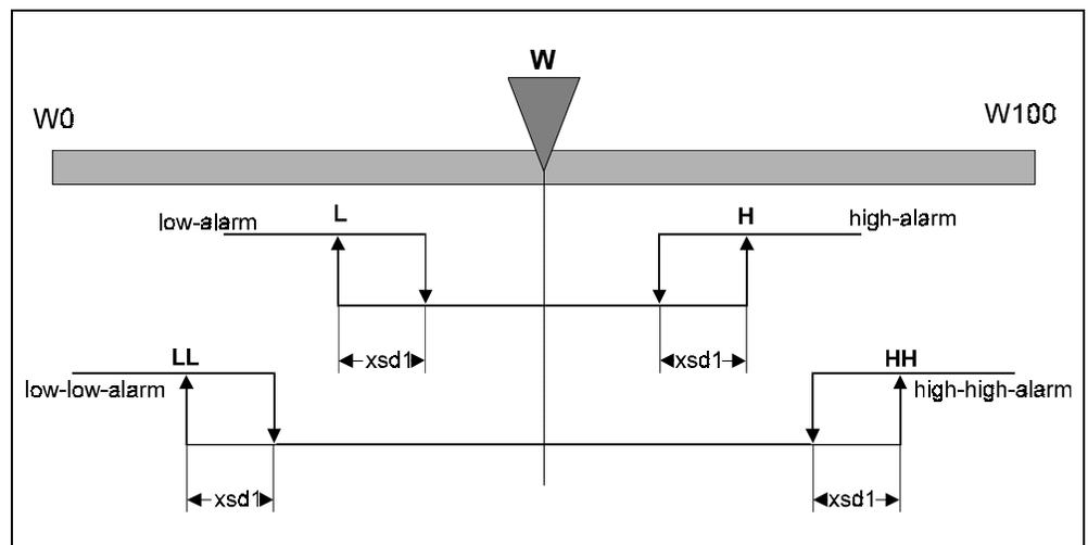
Configuration word C600 and C601 determines which signal shall be monitored by the alarm function and how to use the alarm functions.
